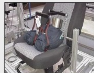
假臀模型模拟座椅 乘员检测试验 Ersatz stern of passenger simulate experimentation
