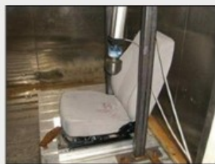
膝压模拟试验 Knee pressure simulate experimentation
