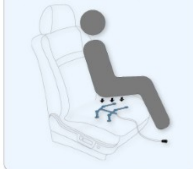
座位传感器结构图 Seat sensors structure drawings
