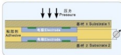
座位传感器结构图 Seat sensors structure drawings
